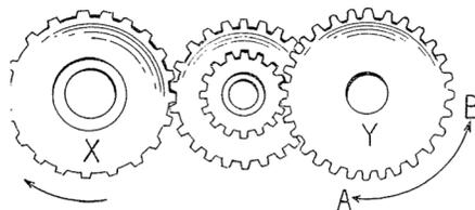
8. When gear X turns in the direction shown by the arrow, gear Y turns
